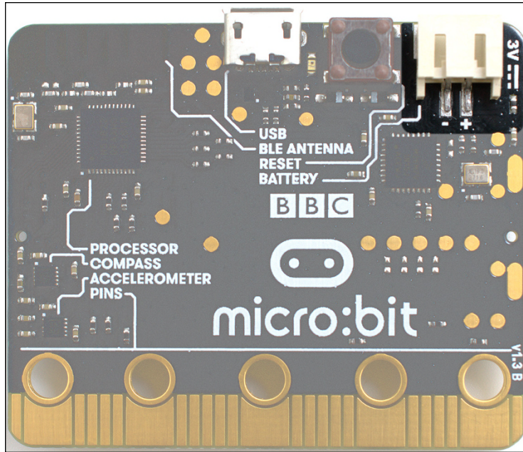
FIGURE 1-11: The BBC micro:bit's battery connector
