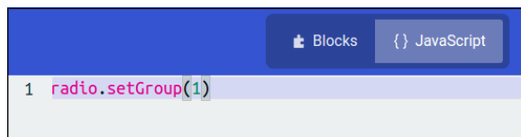
FIGURE 8-2: Setting up the peer-to-peer radio module
