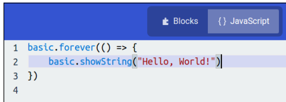
FIGURE 6-5: Looping the basic.showString message
