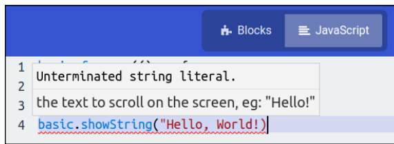
FIGURE 6-3: The JavaScript Editor highlighting a code bug
