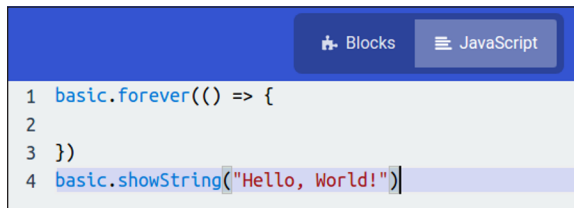
FIGURE 6-2: The basic.showString instruction in the program listing
