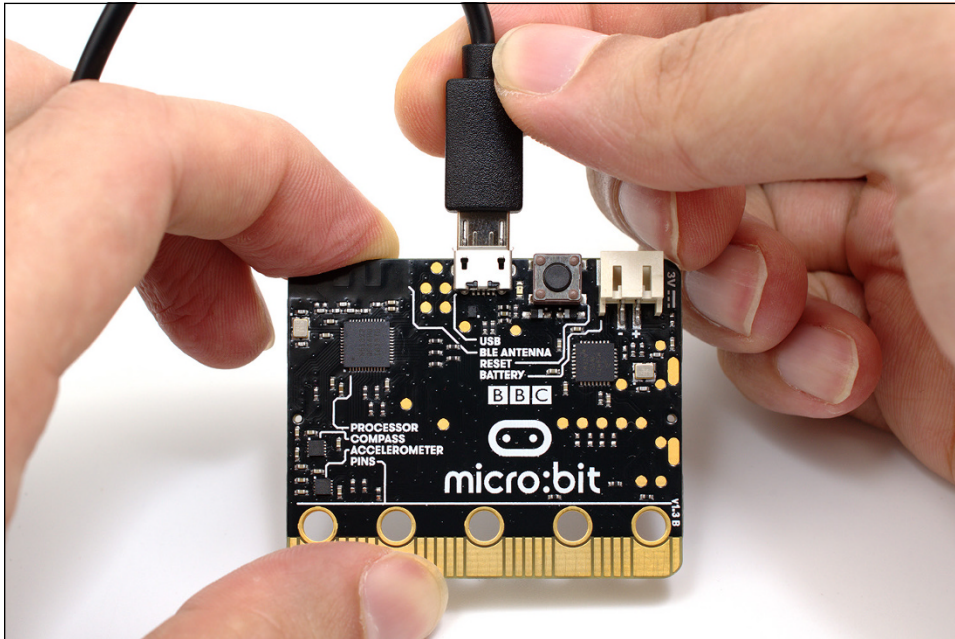
FIGURE 2-1: Inserting micro-USB power
