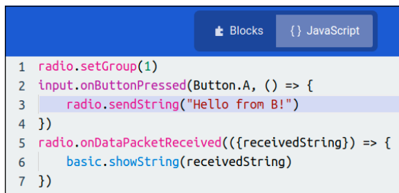
FIGURE 8-4: Modifying the program for a second BBC micro:bit
