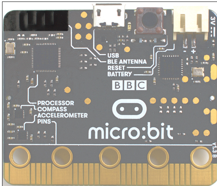
FIGURE 1-6: The BBC micro:bit’s radio antenna
